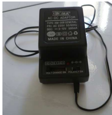
Gambar 7 DC Power Supply
