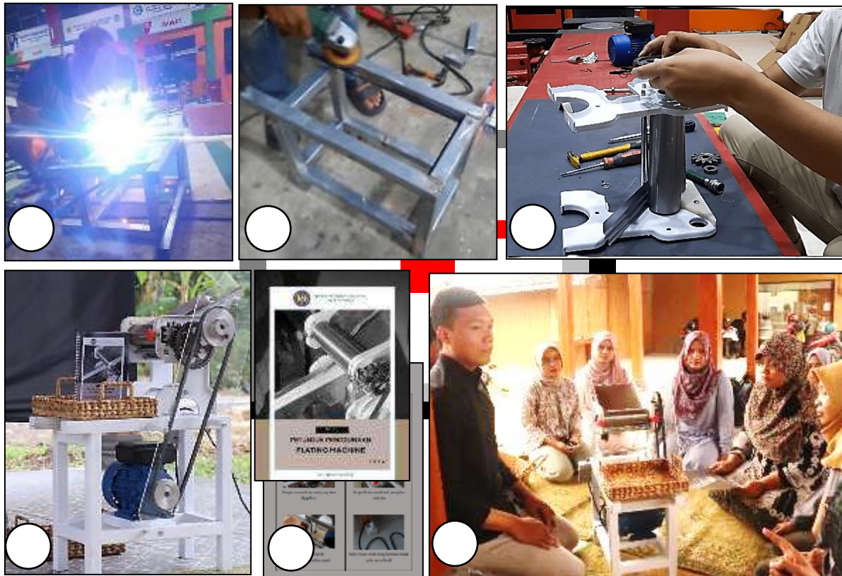
Figure 6. Design Process of Flattening tool, (A) Frame fabrication; (B) Joint grinding; (C) Pressing Roll component connection; (D) Flattening Tool Technology Visualization; (E) User Manual; and (F) Flattening Tool Evaluation and Testing.
