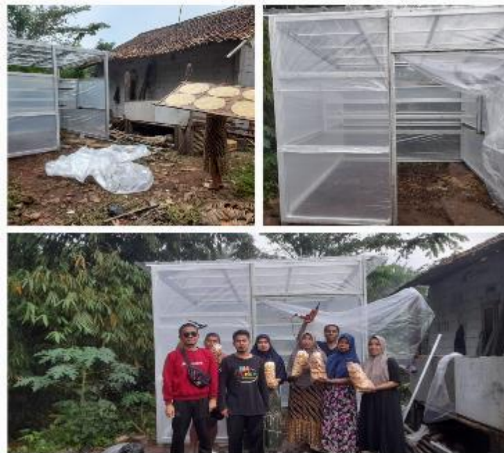
Figure 5. Solar Dome Innovation Technology Application for Drying Opaque Slices
