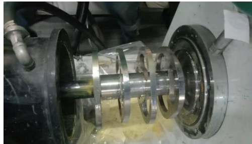
Gambar 3. Pelepasan cover mesin gerinding Horizontal sand mill RTSM-50 ADL E
