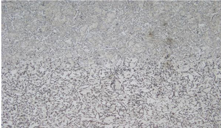
Gambar 12 Struktur Micro 3,2mm Area HAZ Perbesar 200x Etcha Nital 5%
