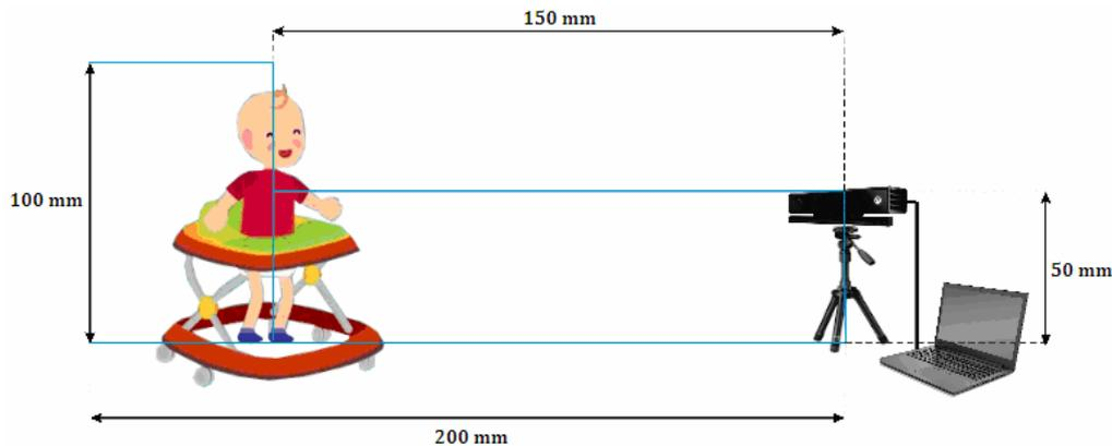
**Figure 1.** Biomechanics Testing Protocol Using Kinect Sensors When Toddlers Push BW
