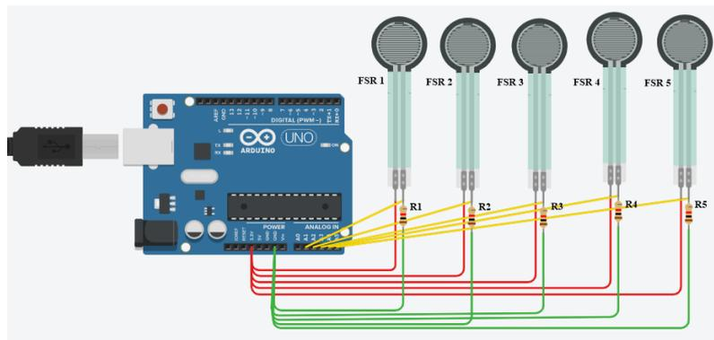
**Figure 5.** Series of Pressure Gauges on The Soles of The Feet
