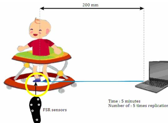
**Figure 2.** Biomechanics Testing Protocol Using The FSR-402 Sensor When Toddlers Push BW
