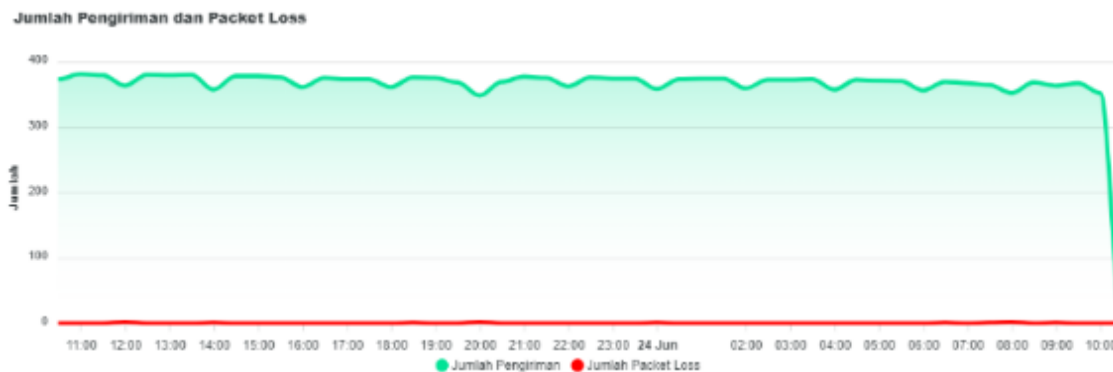
Figure 17. Graph of Transmission Count and Packet Loss Testing on the Third Slave Node
