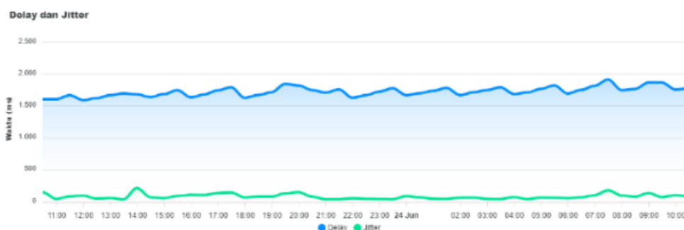
Figure 12. Delay and Jitter Testing Graph on the Master Node
