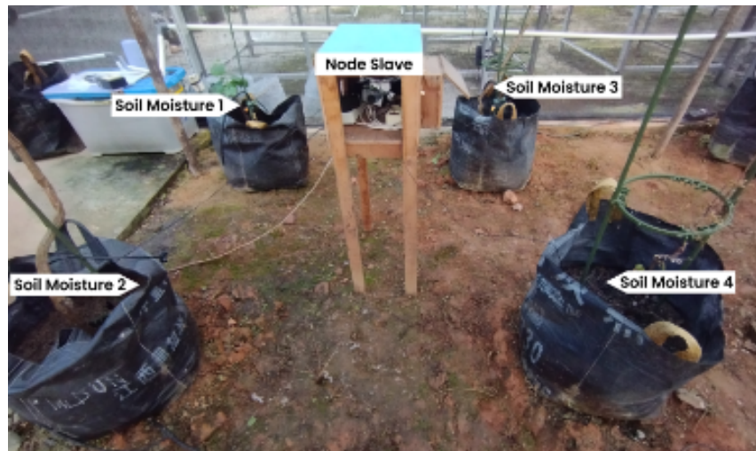
Figure 7. Implementation of the System on Slave Node
